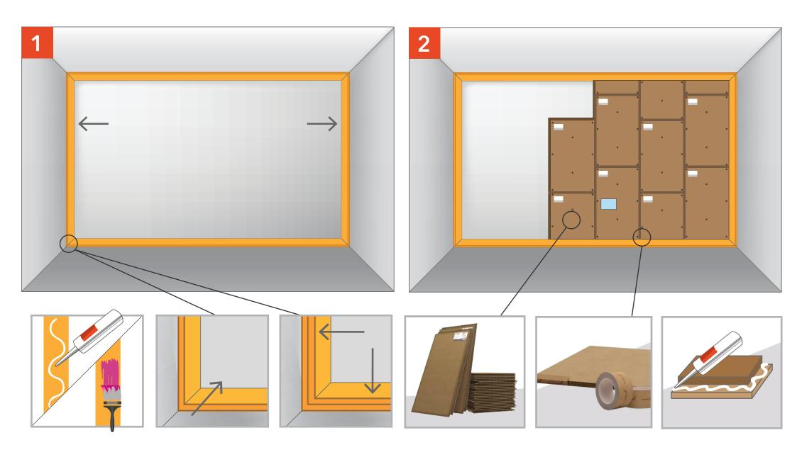
Glue perimeter of the wall with StopZvuk V100 tape using Sonetik sealant or Bautger glue.
