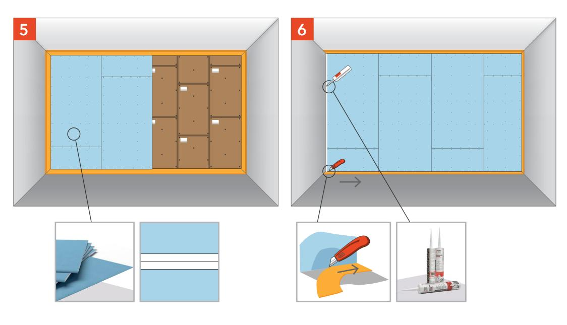
Mount a layer of AcousticGyps GKLZ. Join the sheets horizontally without a gap.
